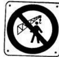
No passage or standing within the crane's radius of action.
